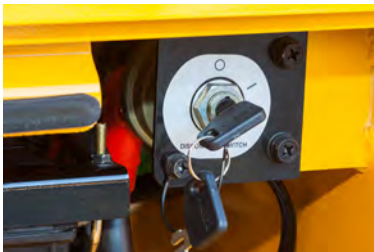
Battery master switch
